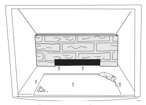
Figure 40. Install Lower Rear Panel
